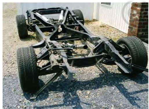
ଚିତ୍ର-୩.୧ : (Chassis With Suspension and Exhaust System )
